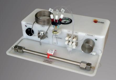
The HPLC+ is a compact system that allows you to add HPLC purification capabilities to any radiosynthesizer which does not have the capability to perform HPLC purification.
