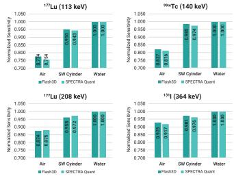
Sensitivity factors obtained as a function of emission energy, phantom geometry, and reconstruction algorithm. Solid Water $^{\text{\tiny M}}$  cylinder proves to be nearly equivalent to use of water-filled IEC body phantom and more practical due to contamination challenges of an IEC phantom.
